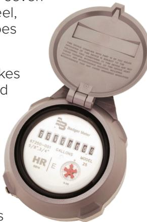
The remaining number slots are white with black numbers (these will correspond to the meter reading indicated on your utility bill). The fourth measures water use in increments of 1,000 gallons, the fifth measures 10,000 gallons, the sixth measures 100,000 gallons, and so on.
