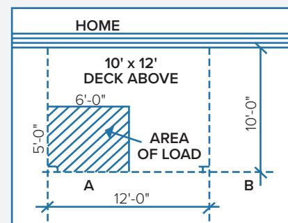
For typical soil conditions, go down the Lbs Supported column until you come to a number larger than 1,500 (in this case 1,605). Read to the left for 14"-diameter size footing.
