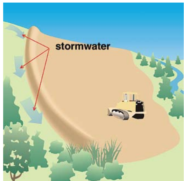
Figure 9. Diversions should be used to divert stormwater away from disturbed areas.
